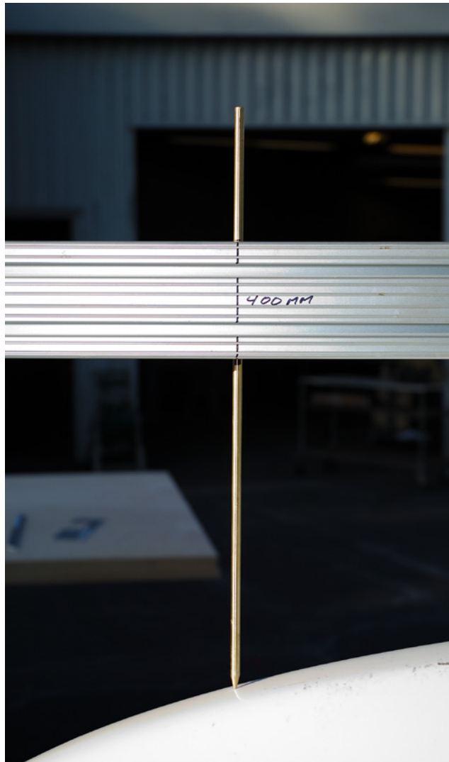
The intersection between the chine extension and the stem head shall be between 311 and 387 mm up from the base line.
